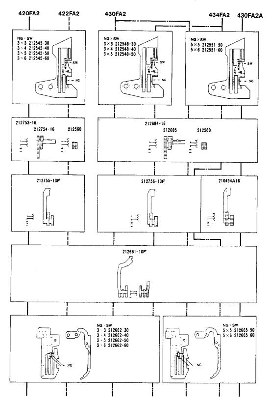
NG=NEEDLE GAUGE SW=SEAM WIDTH
